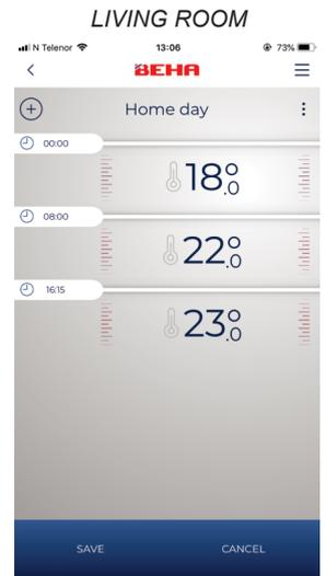
Setting hour and temperature for Home day. Adding times tapping on "⊕". Deleting times by tapping on "⋮" in upper right corner. Tap on **SAVE**. Repeat for Work day and Away day.
