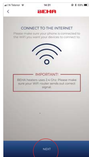
The Wi-Fi on the phone must be switched on and connected to 2,4 GHz. Then tap NEXT .
