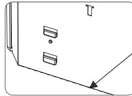
At the bottom of the back plate there are two small triangle tracks. Place the heater onto the tracks and push the heater towards the lips on top of the bracket in an upright position.
