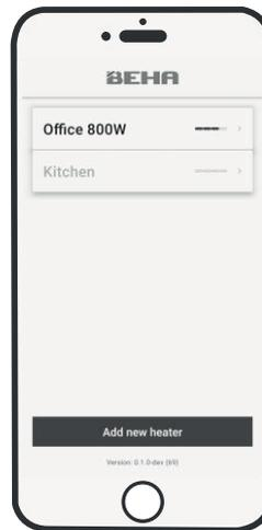
The opening page is showing heaters that are connected to the app. Heaters within range of the phone/tablet will be shown in black, heaters outside of the Bluetooth range will be shown in grey.
